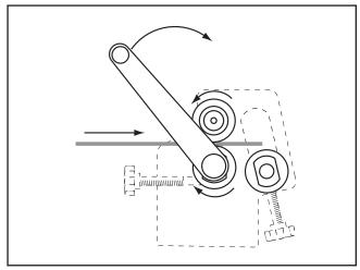
Figure 16. Flat rolling the workpiece.
